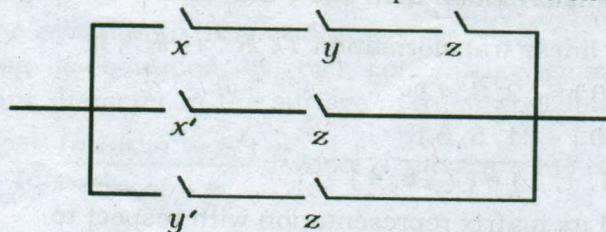
Find a simpler equivalent switching circuit, if any.
